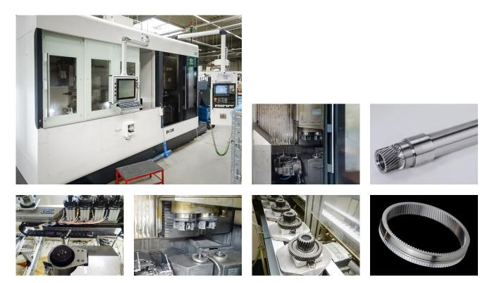
Siemens control system, 8-station tool turret, circulating chain conveyor for parts transport, chip conveyor. Parts conveyor, chip conveyor, manufactured by Kabelschlepp, type Z1705918.1, year 2018, cooling lubricant system. Knoll, type FKA960, year 2017, cooling system, Hyfra
