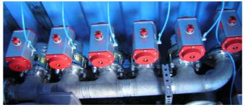
5 electrical-pneumatic valves; 5 tubes out, posibility for rinsing with water
